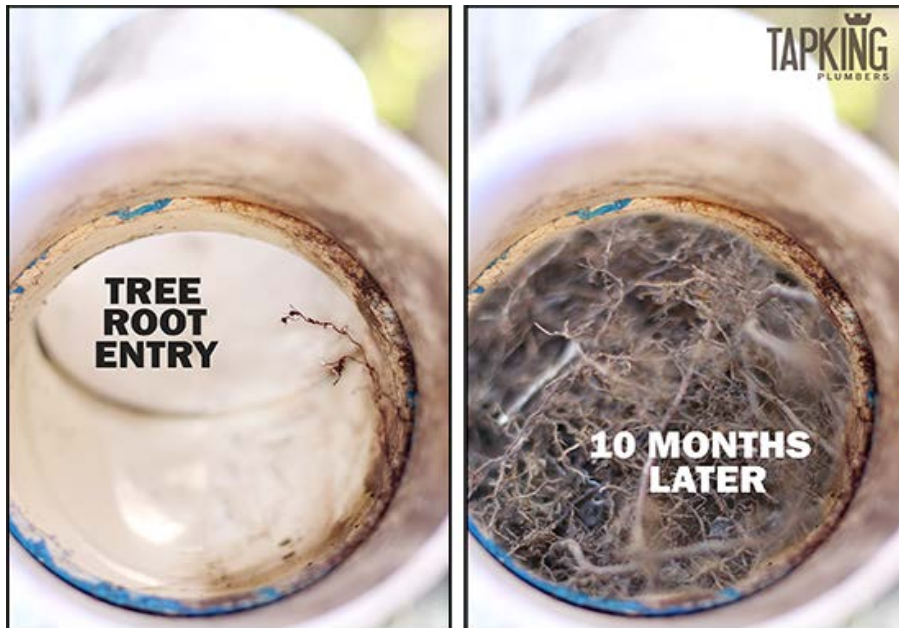
Photo 2 shows a tree root breaking through the walls of a sewer pipe and filling the entire inside within just 10 short months. You can see how this tree root ball does not allow anything to flow past it.
