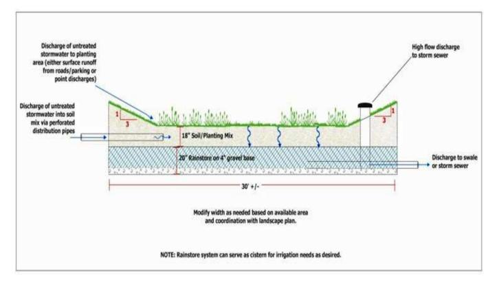
Vegetated Swales with Infiltration Trenches are best fitted for milder sloped swales where the addition of the aggregate bed system is recommended to make sure that the maximum allowable ponding time of 72 hours is not exceeded. This aggregate bed system should consist of at least 12 inches of
