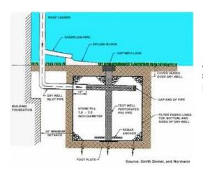
A Dry Well, or Seepage Pit, is a variation on an Infiltration system that is designed to temporarily store and infiltrate rooftop runoff.
