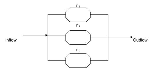
Fig. 8-2. BMPs Connected in Parallel
