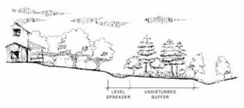
Figure 1.4.2-28 Use of a Level Spreader with a Riparian Buffer Figure 5.3-3 Section of buffer utilization
