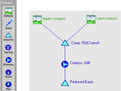
Figure D-1. Model Schematic for Composite BMP
