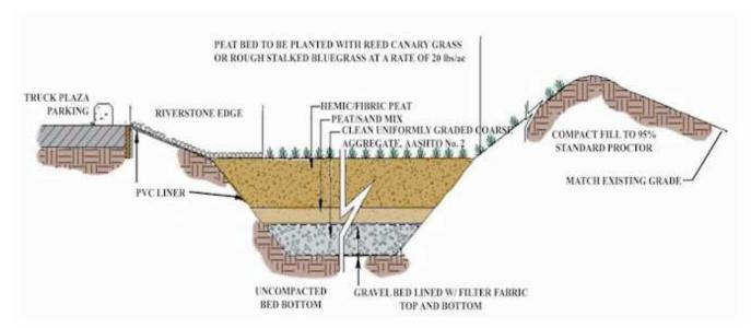
Figure 9-21. Illustrates the peat infiltration bed that is adjacent to the truck parking lot.
