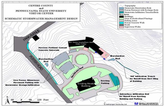
Figure 9-1. Stormwater Management System at PSU Visitor's Center in Centre County, PA.
