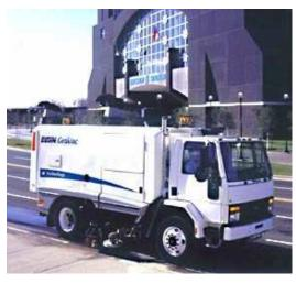
Use of one of several modes of sweeping equipment (e.g., mechanical, regenerative air, or vacuum filter sweepers) on a programmed basis to remove larger debris material and smaller particulate pollutants, preventing this material from clogging the stormwater management system and washing into receiving waterways/waterbodies.
