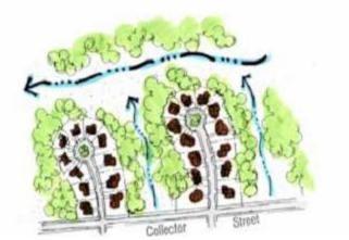
Figure 5.3-5 Natural drainage features can guide the design
