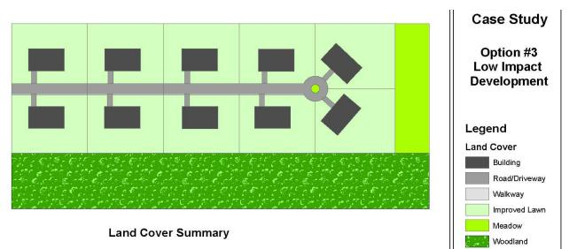
In this example, Woods are maintained, lot setbacks and driveway lengths are reduced, the street width is reduced, and areas of lawn are protected from topsoil
