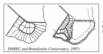
As density is held constant, lot size is reduced, disturbed area is decreased, and undisturbed open space is increased.
