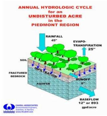
Figure 2-6. Annual hydrologic cycle for an undisturbed acre in the Pennsylvania Piedmont region.
