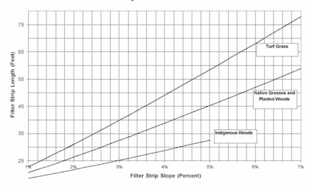
Drainage Area Soil: Sand HSG: A
