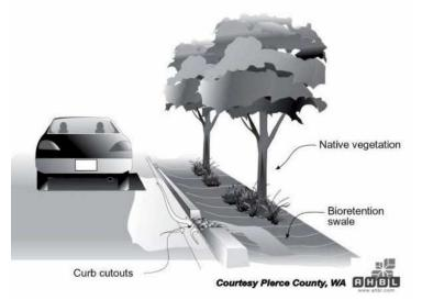
Minimize stormwater volume by disconnecting impervious roads and driveways and directing runoff to grassed swales and/or bioretention areas to infiltrate.
