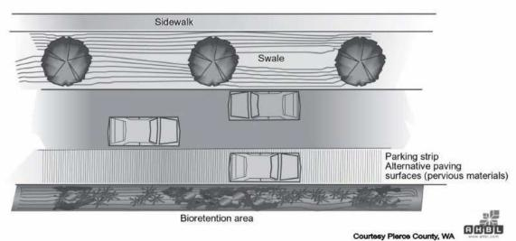
Figure 5.7-1 Reduced road width using adjacent pervious strips.
