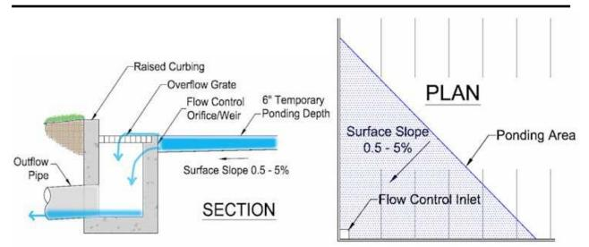
Areas such as parking lots and rooftops that are primarily intended for other uses but that can be designed to temporarily detain stormwater for peak rate mitigation.
