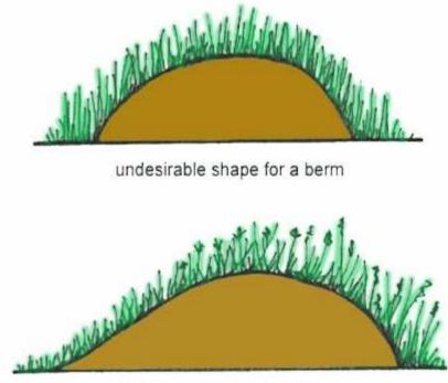
desirable shape for a berm
