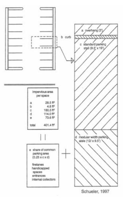
Figure 5.7-5 Parking Stall Dimensions (Schueler, 1997)
