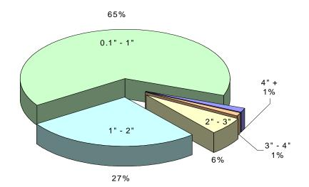
*Figure 2-9. Distribution of precipitation by storm magnitude for Harrisburg, PA (Original Data from Penn State Climatological Office, 1926-2003)*
