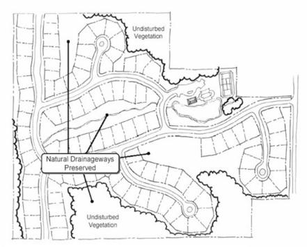
Figure 5.3-1 Protect natural drainage features
