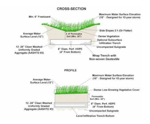
A major concern when designing Vegetated Swales is to make certain that excessive stormwater flows, slope, and other factors do not combine to produce erosive flows, which exceed the Vegetated Swale
