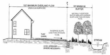
Figure 5.3-2 Section of buffer utilization
