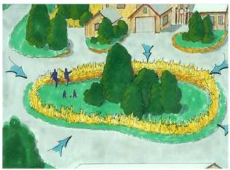
*Figure 5.3-6* Natural surface depressions can temporarily store stormwater.
