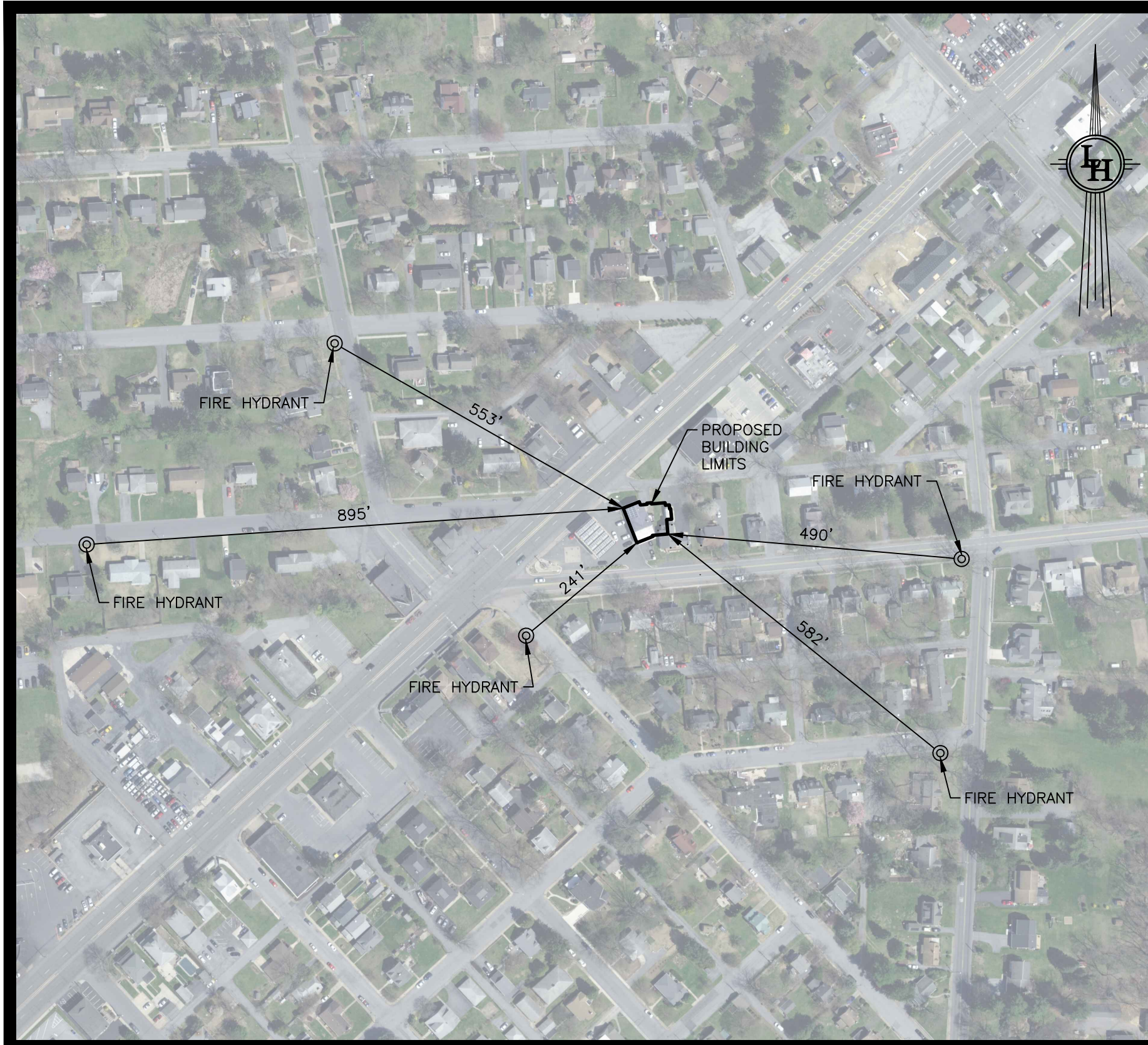
SURROUNDING FIRE HYDRANT LOCATION PLAN
