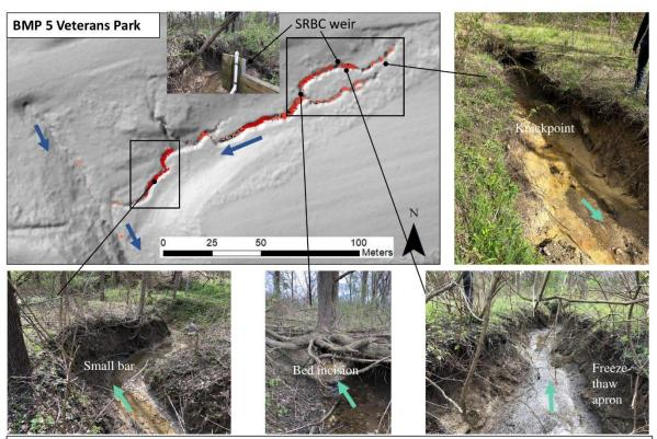
**Figure 3**. BMP 5, Veterans Park, DEM differencing results and field photos from April 29, 2018. Lines indicate field photo sites. Hillshade from 2016 lidar. Inset photo of SRBC weir is facing left bank, in downstream direction.
