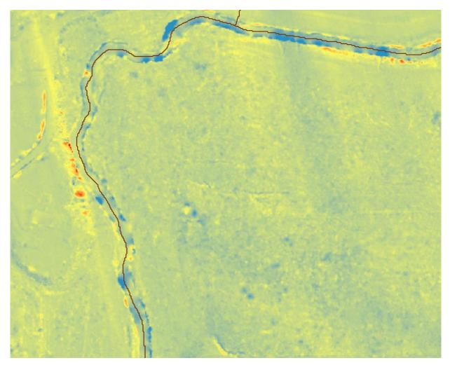
Figure 3. DoD map of Paxton Creek indicating erosion (in blue) and deposition (in red). The site would later be chosen for analysis as BMP-17 utilizing the BANCS method.
