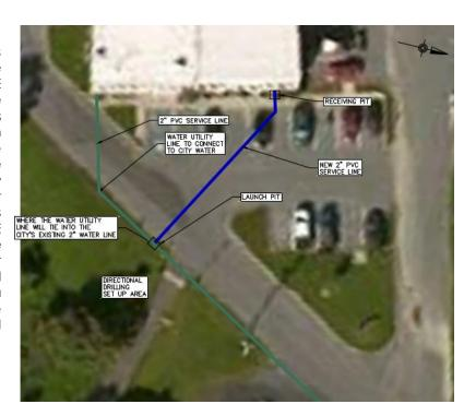
routed through the parking area adjacent to the building. An additional 10-feet of 2-inch HDPE pipe would be used to enter the Maintenance Garage footer and terminate inside the mechanical room. Future plumbing modifications will be needed within the building to connect current mechanical equipment and plumbing fixtures within the building to the new service.
