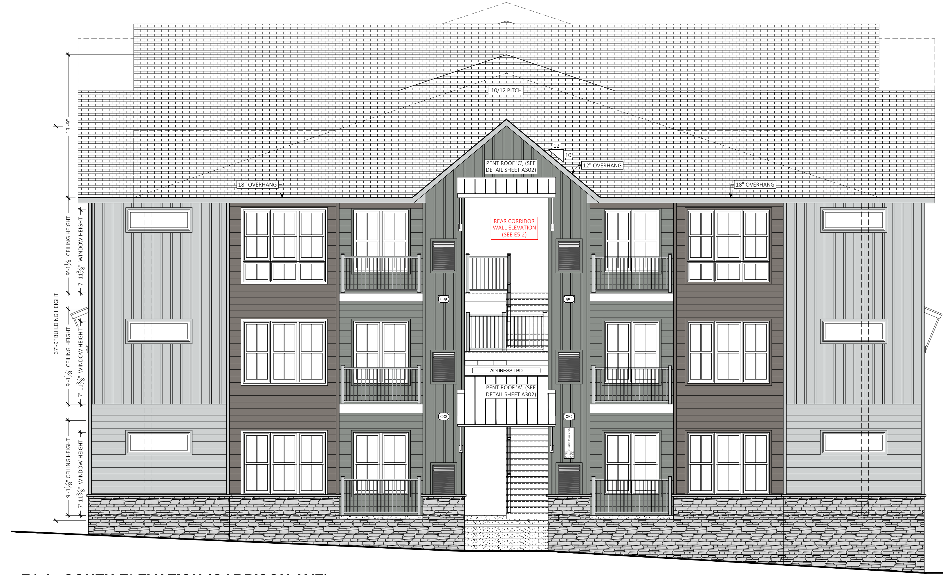
E1.4 - SOUTH ELEVATION (GARRISON AVE) SCALE: 3/16" = 1'-0"
